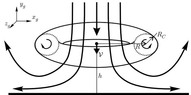
Fig. 4. Wind microburst model
