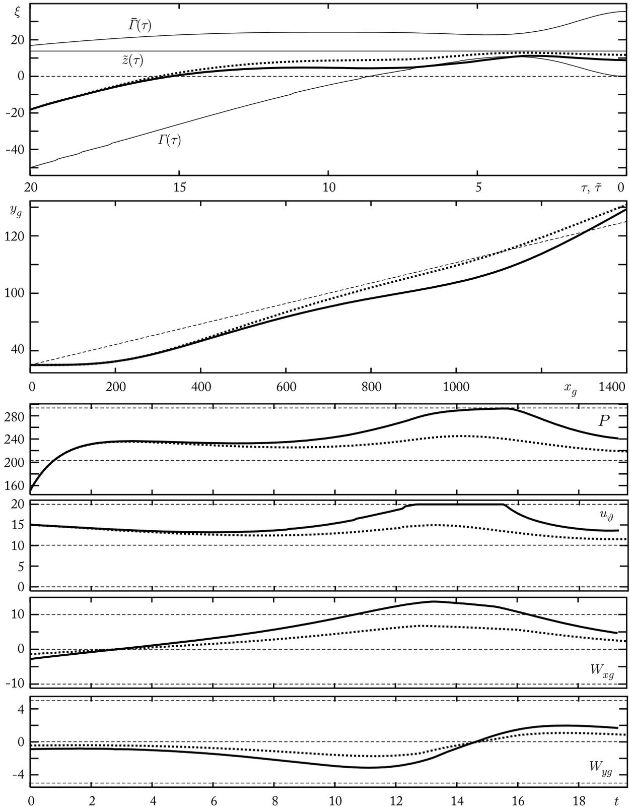
Fig. 5. Simulation results; the plane of auxiliary game (4) in the upper fragment; below that fragment, the graph of the altitude; the graphs of the thrust force  $P$  ( $\times 1000$  N); the prescribed pitch angle  $u_\phi$  (grad); the longitudinal  $W_{xg}$  (m/sec) and vertical  $W_{yg}$  (m/sec) components of the wind velocity
