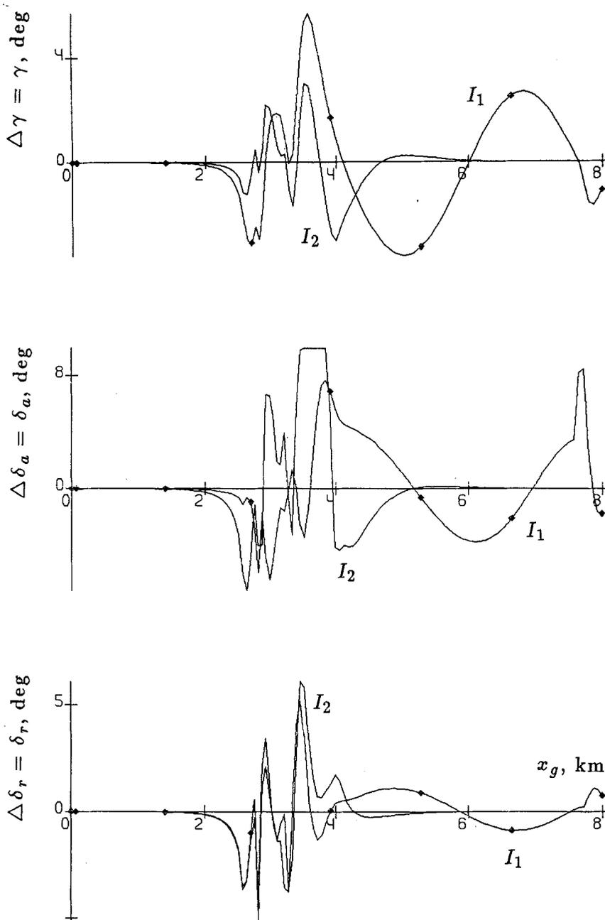
Fig. 7d. Deviation histories: bank angle  $\gamma$ , aileron deflection  $\delta_a$ , rudder deflection  $\delta_r$ ; Model M2, downburst center  $DY = 3000 \text{ m}$ ,  $DZ = 200 \text{ m}$ .
