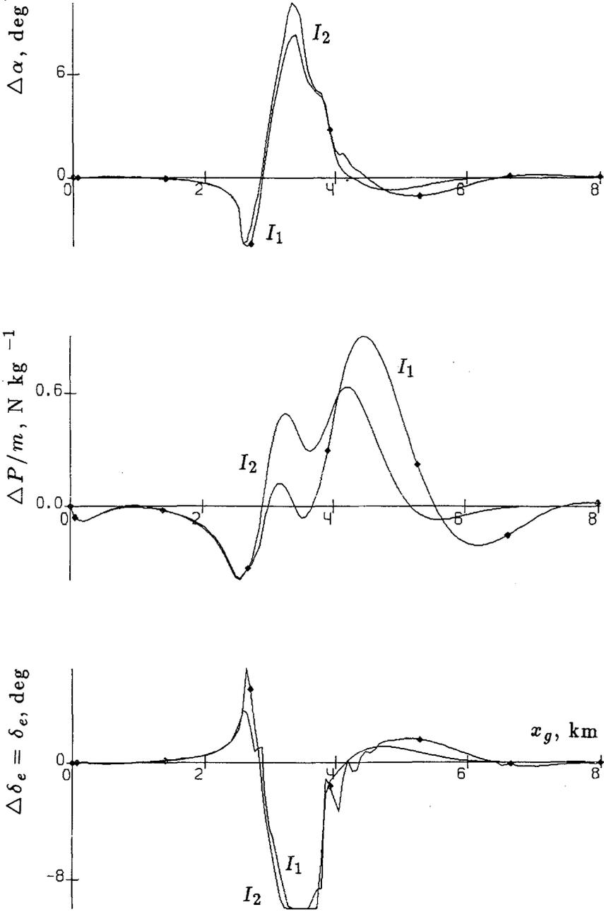
Fig. 7b. Deviation histories: angle attack  $\alpha$ , ratio  $P/m$ , elevator deflection  $\delta_e$ ; Model M2, downburst center  $DX = 3000$  m,  $DZ = 200$  m.
