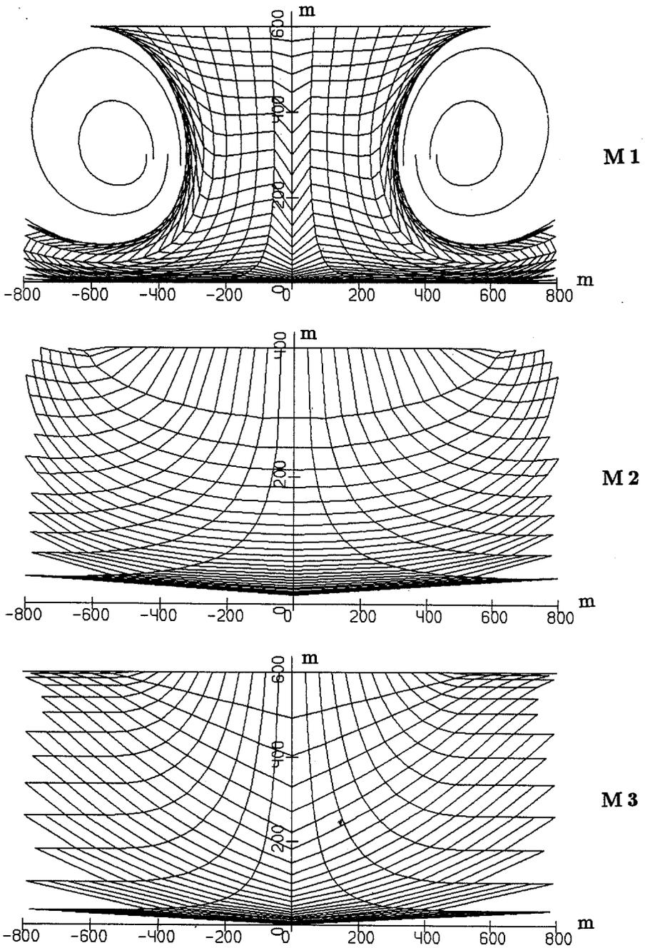
Fig. 3. Downburst models; wind velocity structure in a vertical plane.
