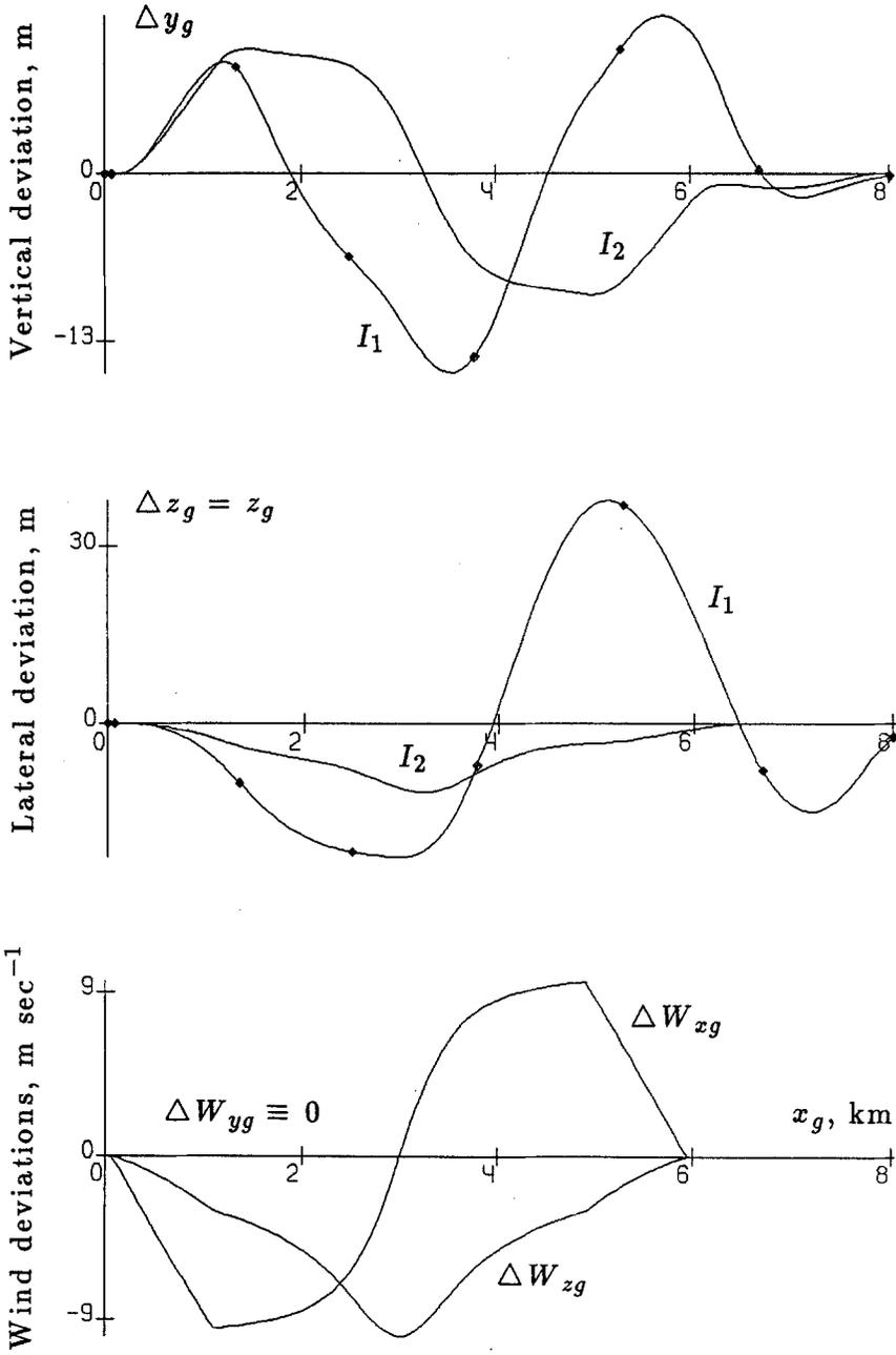
Fig. 6b. Landing simulation results for Model M3; downburst center  $DX = 3000$  m,  $DZ = 600$  m.
