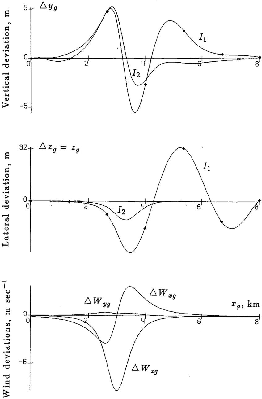
Fig. 5b. Landing simulation results for Model M2; downburst center  $DX = 3000 \text{ m}$ ,  $DZ = 600 \text{ m}$ .
