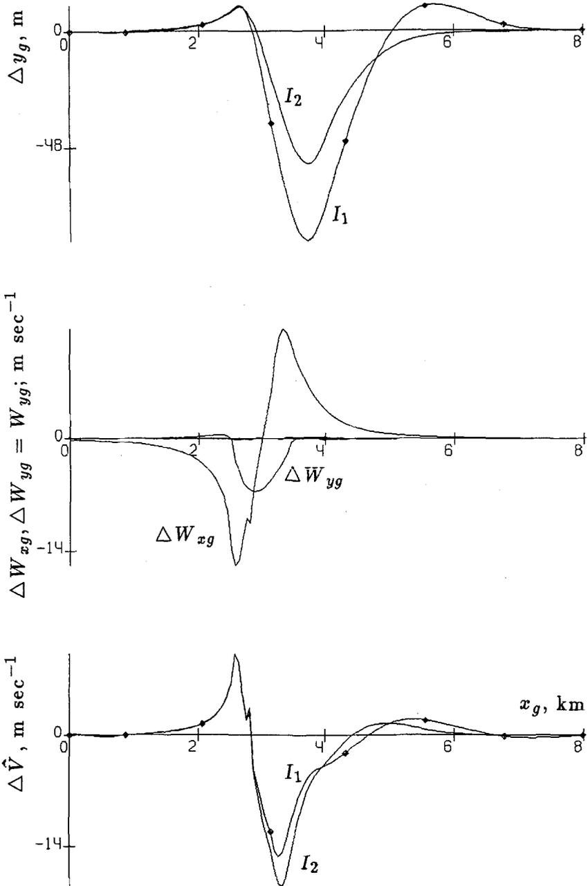
Fig. 7a. Deviation histories: altitude  $y_g$ , wind velocity components  $W_{xg}$  and  $W_{yg}$ , relative velocity  $\hat{V}$ ; Model M2, downburst center  $DX = 3000 \text{ m}$ ,  $DZ = 200 \text{ m}$ .
