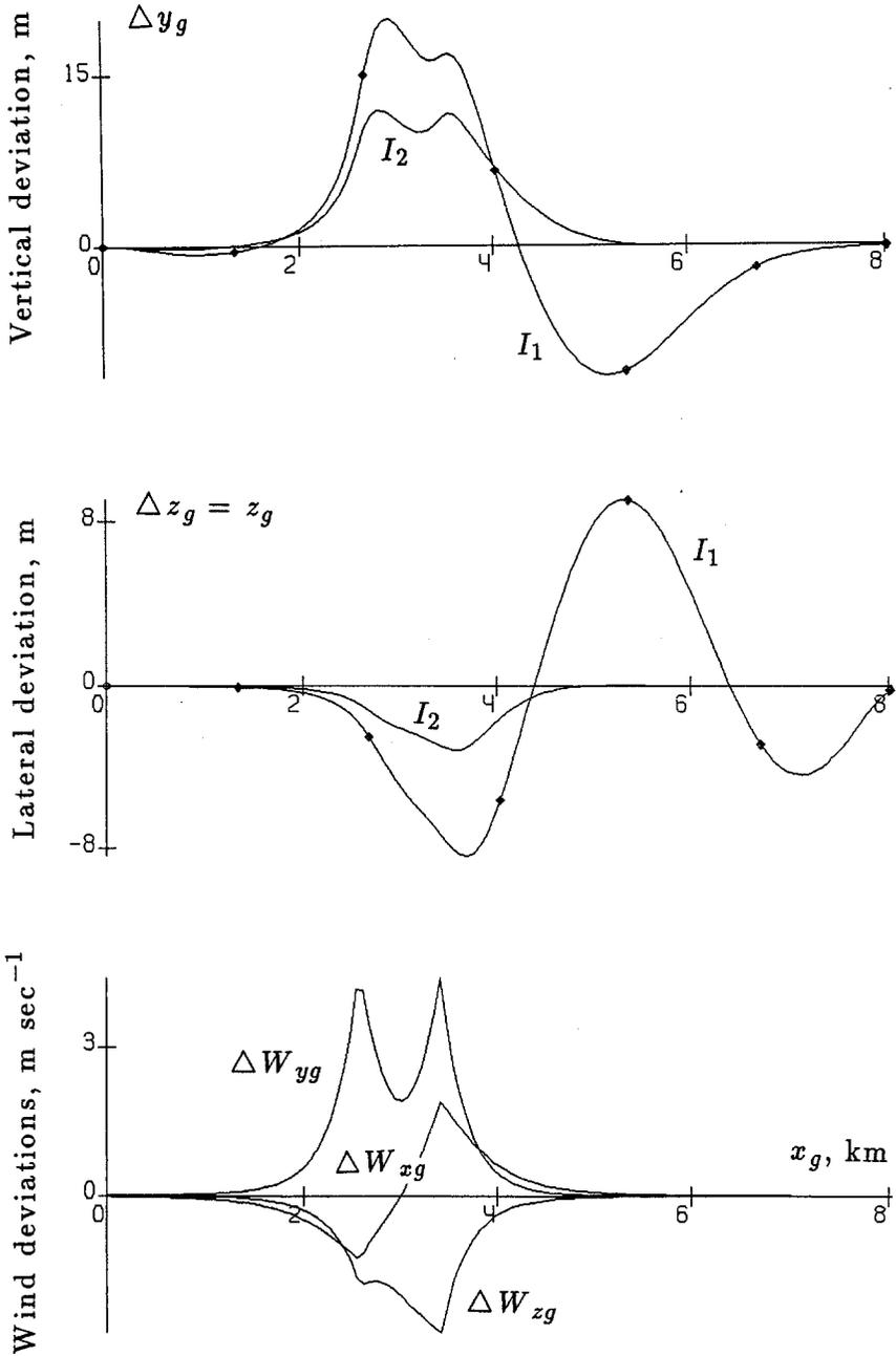
Fig. 4b. Landing simulation results for Model M1; downburst center  $DX = 3000$  m,  $DZ = 600$  m.
